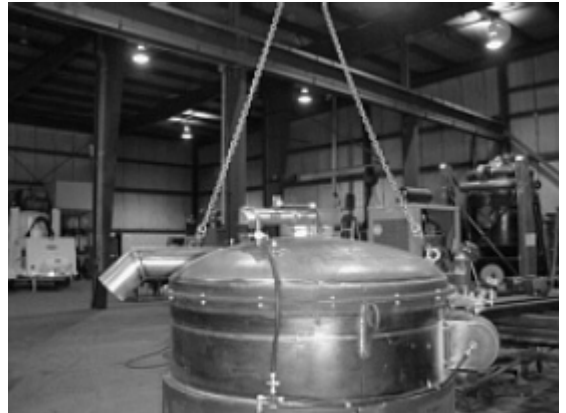
Filter Fig. 5 Lifting chains attached to lid eyes.
