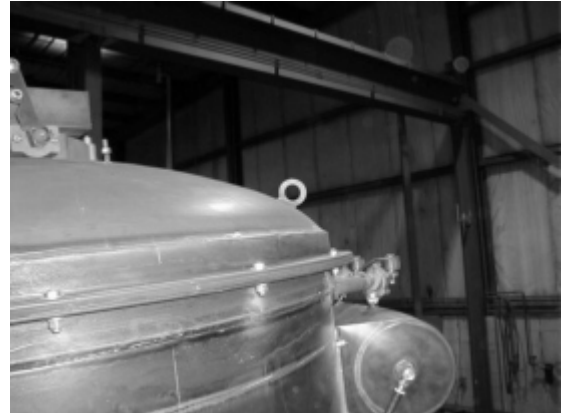
Filter Fig. 3 Remove all bolts on lid flange. Disconnect the air line and the power supply wire to the air cylinder.
