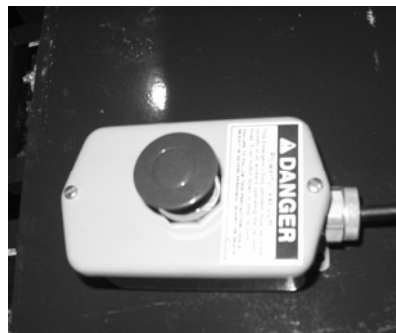
Figure 7. Remote shut down button
