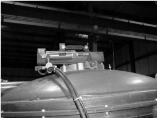
Filter Fig. 4 Butterfly valve and air cylinder with rain cover removed.
