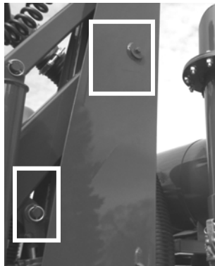
Figure 12. Lift Arms- 10 grease points
