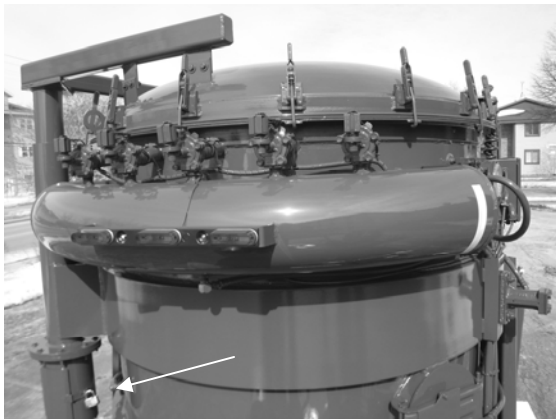
Filter Fig. 4 Butterfly valve and air cylinder with rain cover removed.
