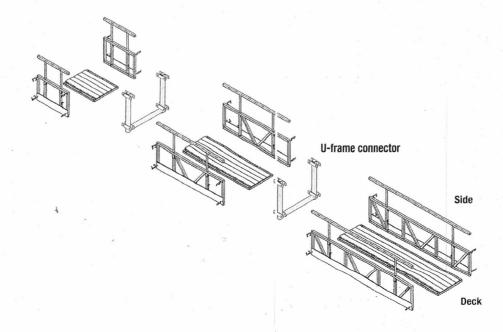
U-Frames (PMR0041C) can be used in place of 4-H bracket to connect sections
