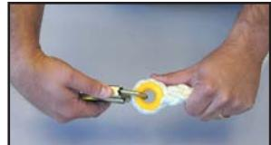
• Thimbles: The thimble must be firmly seated in the eye of the splice, and the splice should have no loose or cut strands. The edges of the thimble must be free of sharp edges, distortion, or cracks.
