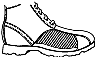
Figure 14. Steel-Toed Boots (sectioned)
