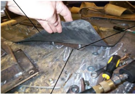
Tapered edge on Main Seal Main Seal
