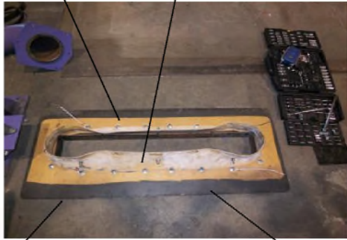
Tapered edge on Main Seal Main Seal
